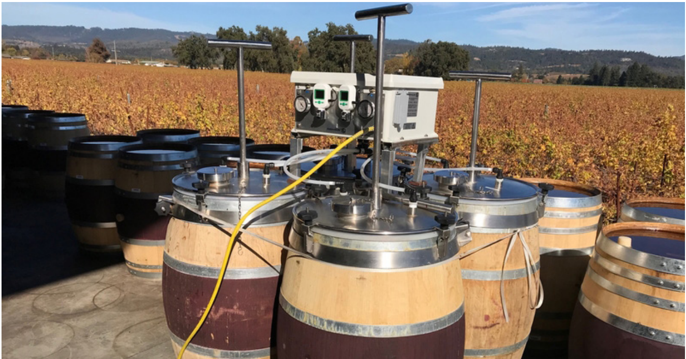
Malbec was fermenting Tuesday at Alpha Omega in barrels equipped with an AromaLoc machine. The seal was designed by barrel producer TN Coopers of Chile. Photo by Kerana Todorov/Wine Business Monthly
