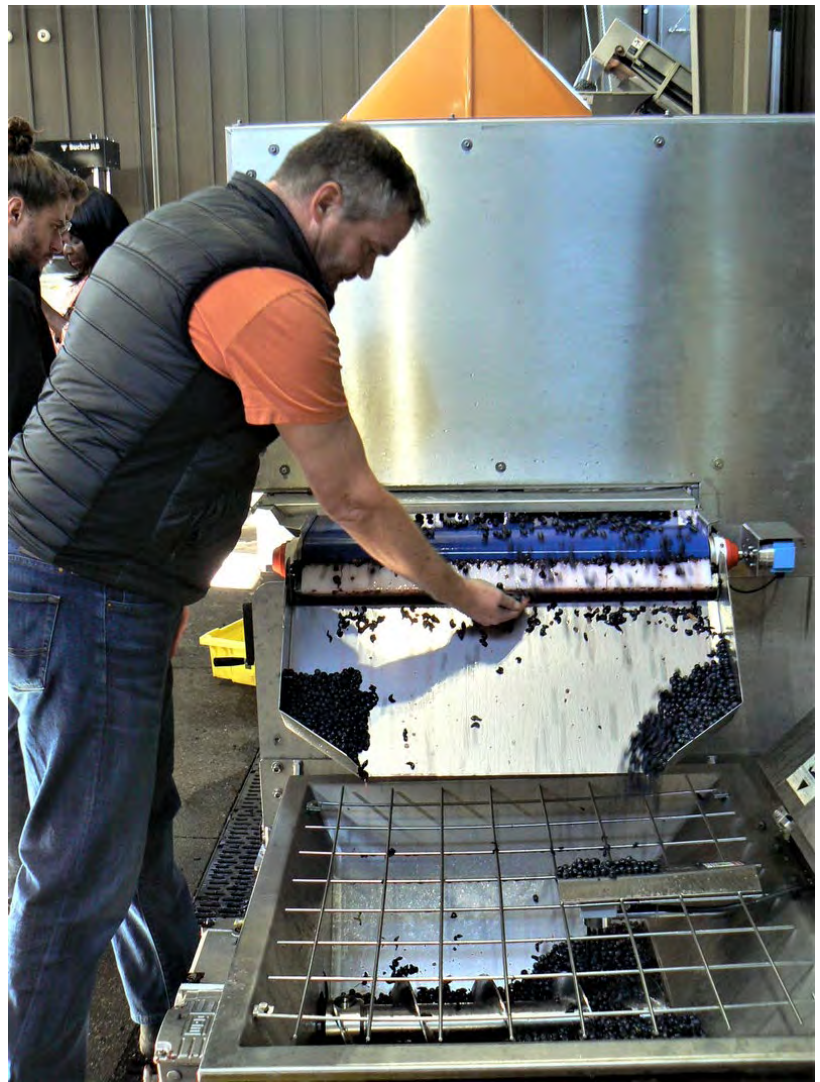
Alpha Omega winemaker Jean Hoefliger inspects sorted berries coming off Alien sorter conveyor
